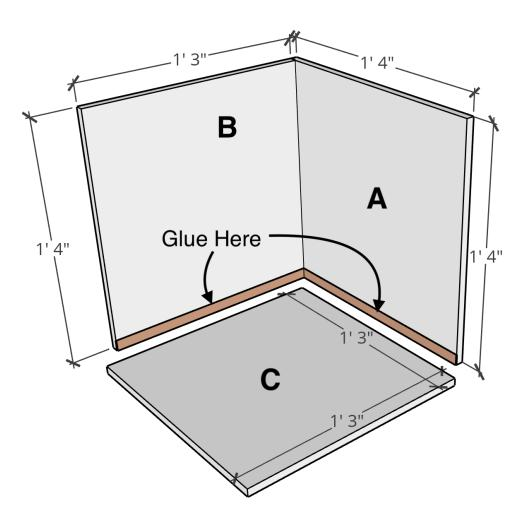
4. Staple through the outsides of panels A and B into the edge of panel C. If you have a reliably flat work surface, you can move the piece to the edge of your surface and use it as a guide to ensure that the pieces remain properly flush while stapling. If not, I would recommend rotating the piece as you work so that you have a clear view of how the panels are lining up as you attach them to each other.
