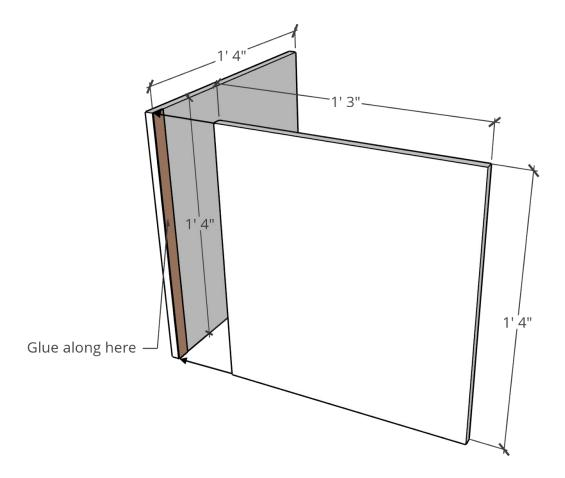
2. With the two pieces fitted flush to each other, make sure that the edges are also flush, and then staple or screw through the face of panel A into the edge of panel B.
