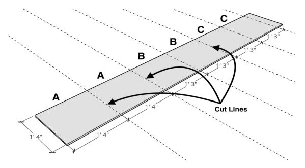
Note about cut C: This will be a two-part cut. First you will cut the pieces at 1'-4" x 1'-3", then you will cut an additional 1" to create a finished square of 1'-3" x 1'-3" that matches the cuts made to the B sides of the cube.
