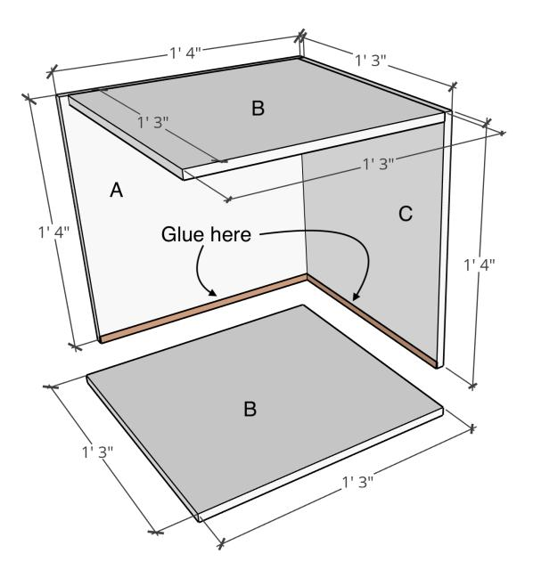
6. Glue along the exposed edges of the box, and place and staple the final panel A piece into place.
