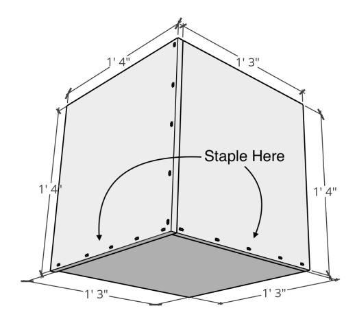
5. Flip the piece over, glue along the inside edges of the corner pieces, and fit the other panel B into the corner then staple along the outside edges in the same way as step 4.
