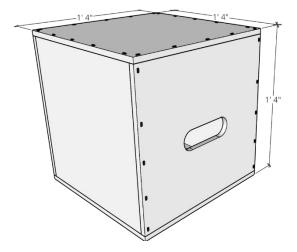
Optional: You may want to use wood cleats to better secure the edge joints and compensate for the potential loss of strength associated with joining plywood along its edge. Cut cleats from scrap (1"x1"x4") and place them along the inside edges of the cube as you're assembling it. They should be glued and fastened as you would with the rest of the cube.
